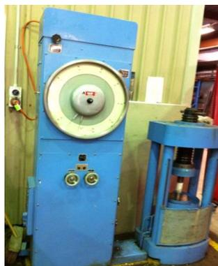
Figure 2 - Uniaxial compressive test set-up
