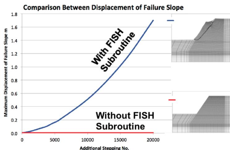
Figure 7 - Comparison between slope displacement at failure for FLAC model with and without application of FISH subroutine
