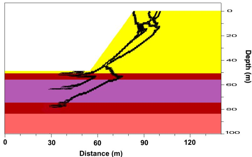
Figure 6 - Simulated failure in unsupported rock slope
