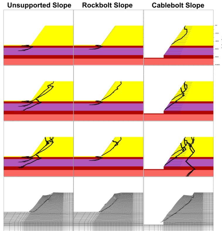
**Figure 8 - Comparison of simulated rock slope progressive failure**
