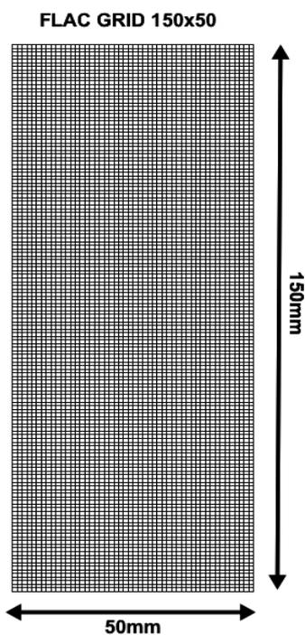
**Figure 2 - FLAC model geometry for cylindrical rock**
