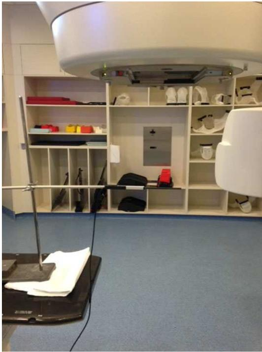
**FIG. 3.** Experimental setup for the measurement of  $CTDI^{in-air}$ . The 100-mm chamber was stepped in 100-mm increments to achieve the necessary integration length to capture the full dose profile. The chamber was held in place using a retort stand and rod. The chamber was extended from the couch a distance equal to half the total integration length to minimize scatter from the couch as specified by the IAEA.<sup>15</sup>
