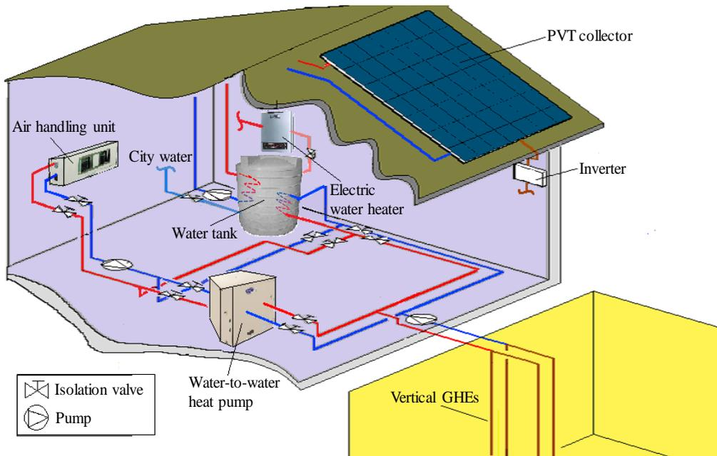
Fig. 1 Schematic of the proposed GSHP-PVT system.
