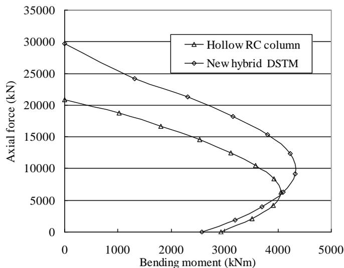
**Figure 3 - Axial force-bending moment interaction diagram**
