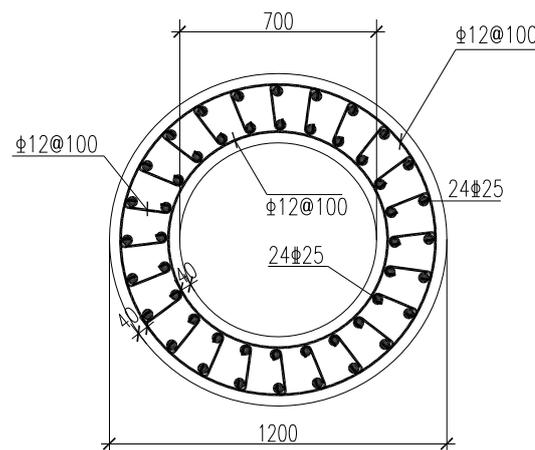
Figure 2 - Cross-section of hollow RC column
