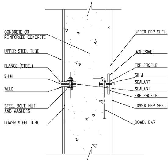
**Figure 8 - Segmental construction of hybrid DSTMs**
