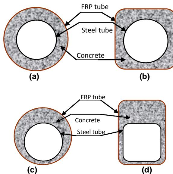
Figure 1 - Typical sections of hybrid DSTMs
