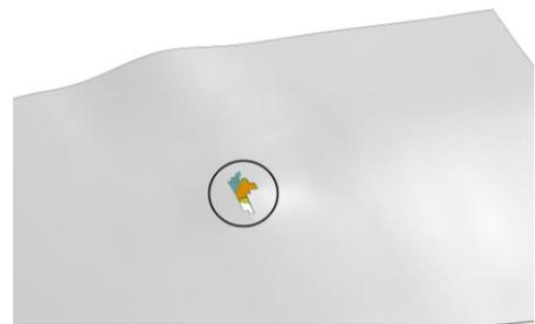
**Figure 20 - Perforation of steel cover plate**
