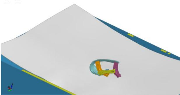
**Figure 19 - Large deformations of wall bracket**
