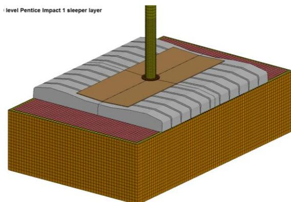
Figure 8 - 9 level pentice impact model
