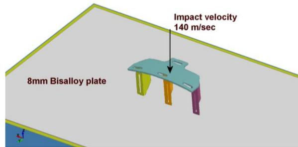
**Figure 18 - Model of wall bracket impacting pentice structure**
