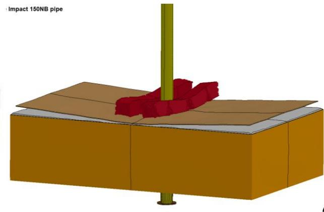
Figure 11 - Effect of single layer of sleepers
