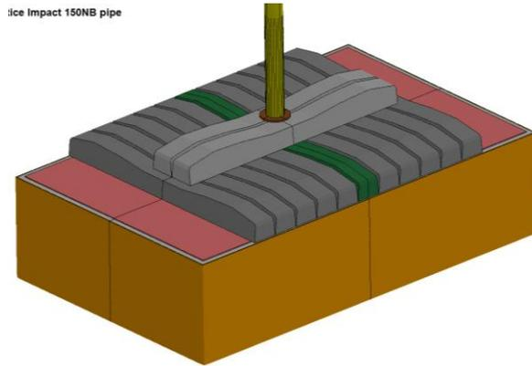
Figure 4 - Two layers of sleepers protection
