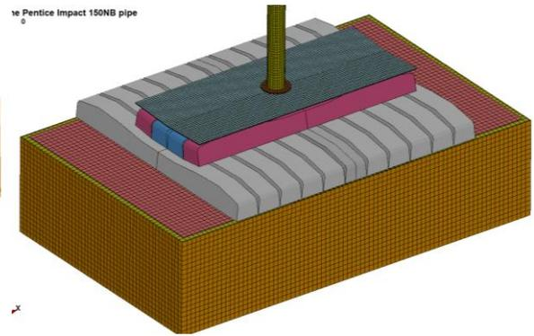
Figure 5 - Concrete sleepers and steel plate
