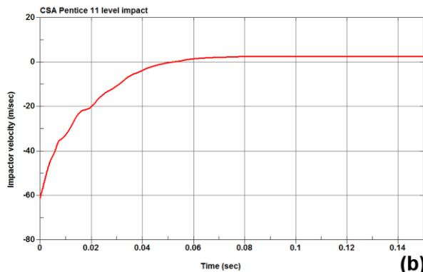
Figure 14 - Response of 11 level pentice
