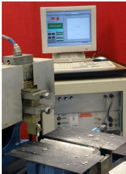
Figure 2 - Instrumentation used in the core cuttability test procedure at UNSW
