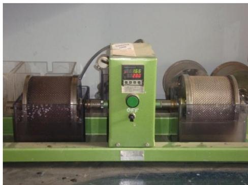
Figure 1 - Slake durability index test apparatus
