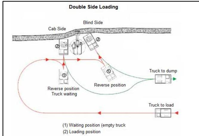
Figure 2 - Double-side truck loading (Fiscor, 2007)
