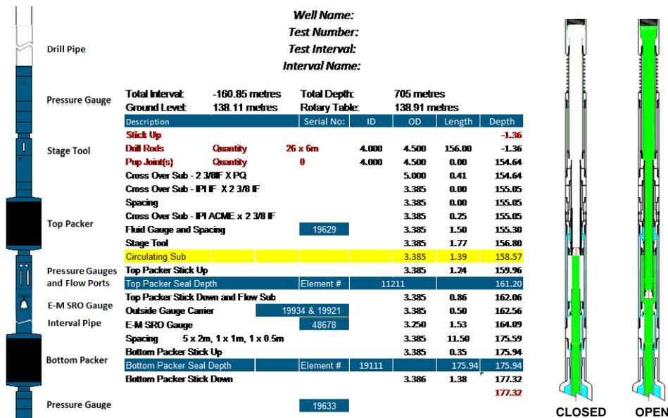
Figure 1 - Tubing pressure actuated DST system
