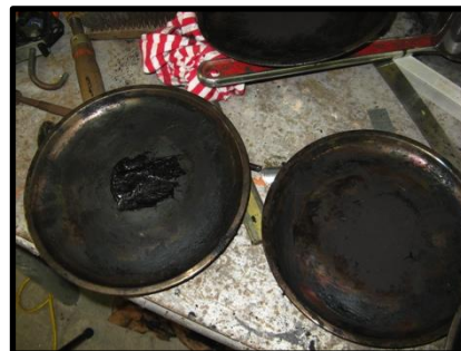
Figure 2 - Simulated bearing housings with surface coal and grease
