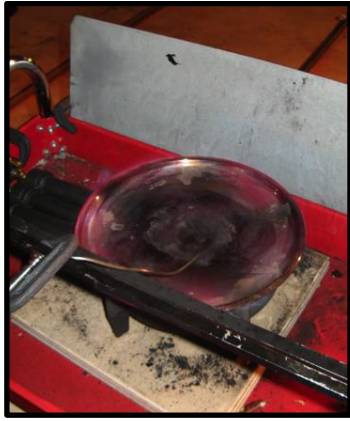
Figure 3 - Heated simulated bearing housing without fuel
