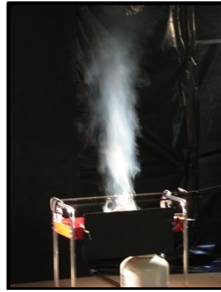
Figure 4 - Typical smoke plume resulting from heating the coal and grease fuel mixture
