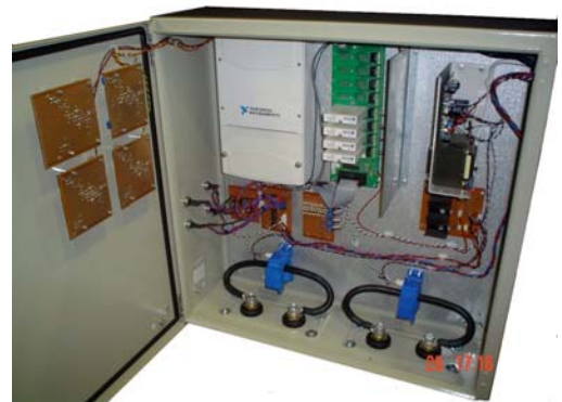
Figure 5. Test System DAQ and Sensor Enclosure
