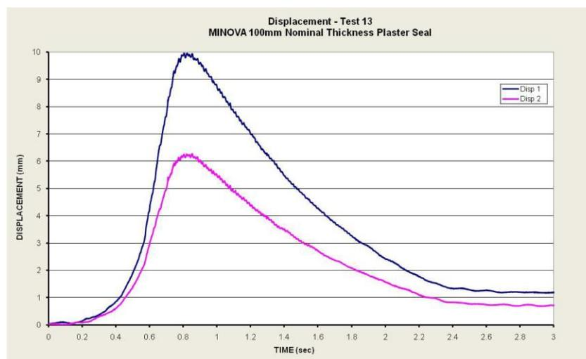
**Figure 7 - Seal displacement versus time in Test 13**
