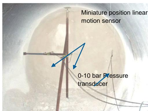
**Figure 5 - Layout of instruments for measuring structural response**
