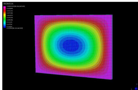
Figure 12- Peak mine seal deflection during a blast
