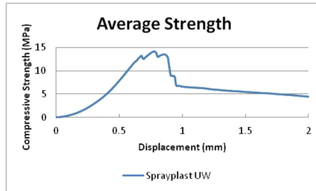
Figure 1 - Compressive strength versus displacement
