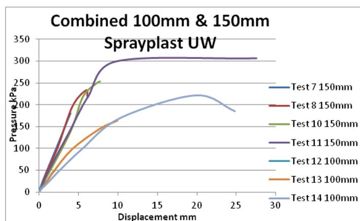
Figure 8 - Pressure versus displacement at seal centre
