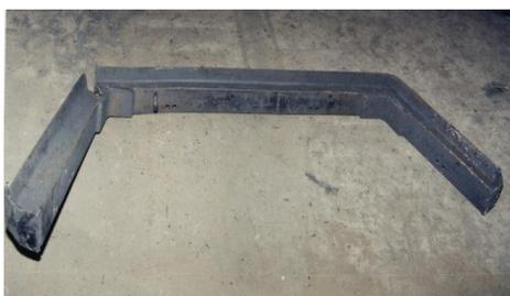
Figure 2 - Support crater cracking
