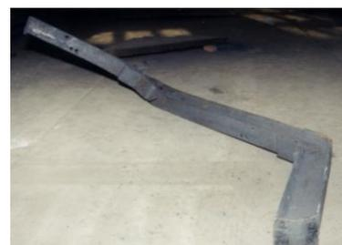
Figure 3 - Support twist and deform
