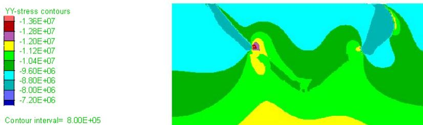
Figure 8 - Vertical stress distribution after coal mining
