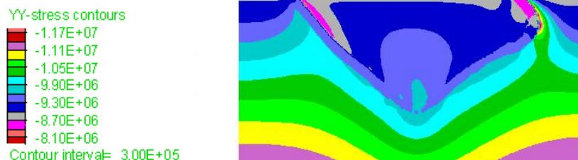
Figure 7 - Vertical stress distribution before coal mining
