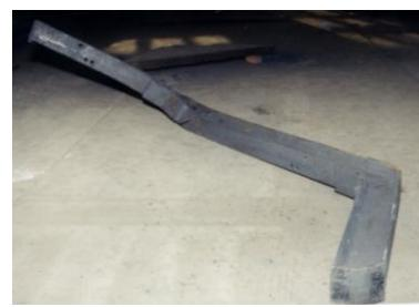
**Figure 3 - Support twist and deform**
