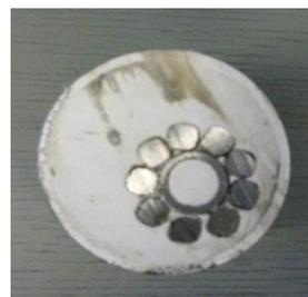
Figure 4 - Cross-section of 8 m Megadowel
