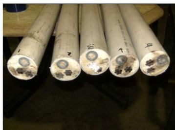
Figure 3 - Cross-section of 6 m twin strand cables
