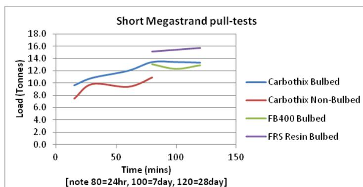
**Figure 10 - Pull test results with pull duration**
