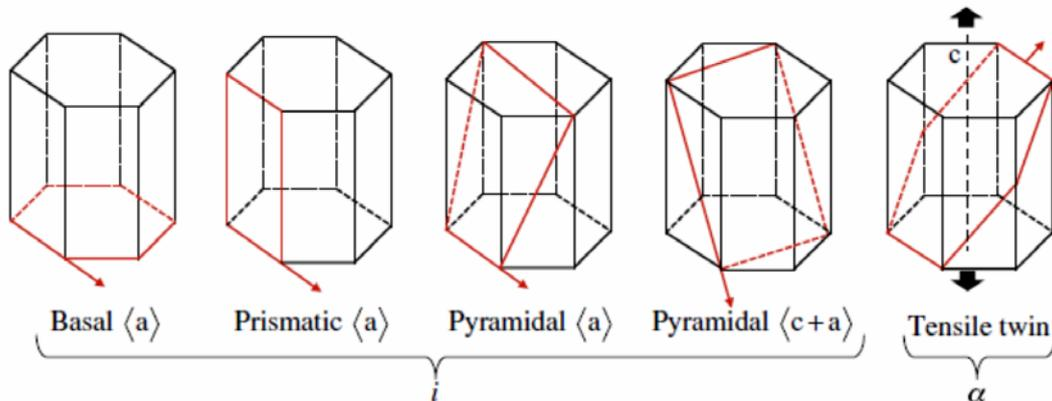
Figure 2 Schematic of the four hcp slip system (i) considered here, along with the tensile twinning system (a) [18]
