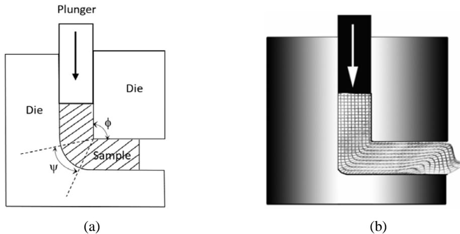
Figure 4. Schematic of ECAP process: (a) ECAP device (die, punches and sample), (b) simulated sample deformation by FEM [33]
