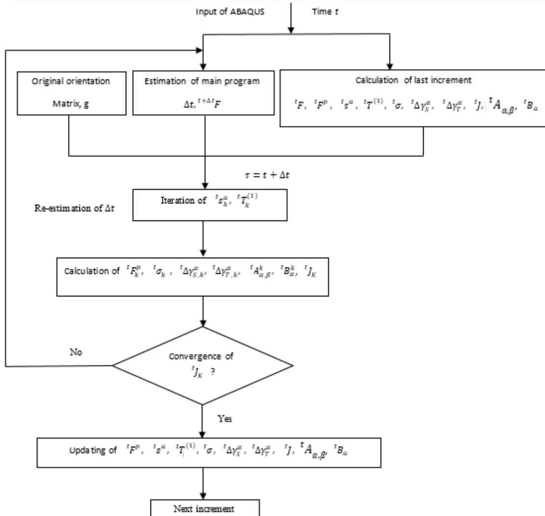
Figure 6 Flowchart of the UMAT code of HCP metal (Mg alloy) used in ABAQUS
