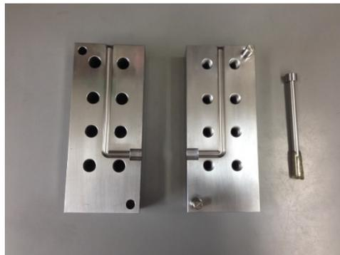
Figure 3 Micro-ECAP device: dies and punch
