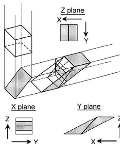
Figure 5. Schematic illustration of shearing in a single pressing through the die: X, Y and Z define orthogonal planes of observation [34]
