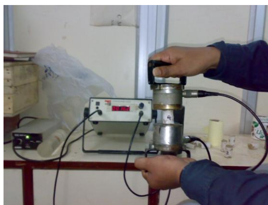
Figure 2 - P-wave velocity determination of sandstone samples from Laboratory testing
