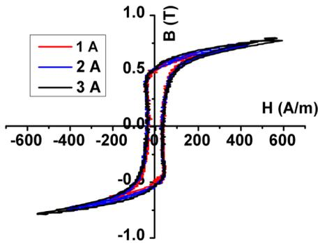
FIG. 5. Measured  $B$ - $H$  curves at  $40^\circ\text{C}$ : maximum magnetic flux density at 1, 2, and 3 A is 0.65, 0.74, and 0.80 T, respectively.
