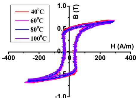
FIG. 6. Measured  $B$ - $H$  curves at different temperature ranging from  $40^\circ\text{C}$  to  $100^\circ\text{C}$ : maximum magnetic flux density at  $40^\circ\text{C}$ ,  $60^\circ\text{C}$ ,  $80^\circ\text{C}$ , and  $100^\circ\text{C}$  is 0.65, 0.65, 0.64, and 0.63 T, respectively.
