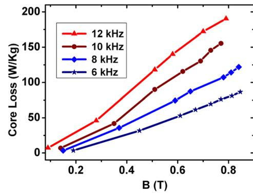
FIG. 7. Measured core losses at different frequency ranging from 6 kHz to 12 kHz; experiments were carried out at  $40^\circ\text{C}$ .
