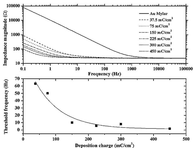
**Fig. 5** (a) Impedance magnitude of PPy/GG electrodes as a function of perturbation frequency for deposition charges between  $37.5 \text{ mC cm}^{-2}$  and  $450 \text{ mC cm}^{-2}$ . The impedance of an uncoated Au Mylar electrode is shown for comparison. (b) The threshold frequency value (where impedance magnitude becomes independent of frequency) for PPy/GG coated electrodes prepared using  $0.25 \text{ mA cm}^{-2}$ . The solid line is an exponential fit to the data ( $R^2 = 0.93$ ).
