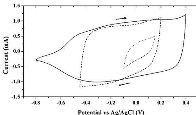
**Fig. 6** Cyclic voltammograms of PPy/GG coated electrodes prepared using  $150 \text{ mC cm}^{-2}$  deposition charge. Large ( $-0.80$  to  $+0.40 \text{ V}$ , solid line), medium ( $-0.45$  to  $+0.20 \text{ V}$ , dashed line) and small ( $-0.10$  to  $0.15 \text{ V}$ , dotted line) potential ranges were explored. Scans were obtained at  $100 \text{ mV s}^{-1}$  starting at the negative end of each potential window.
