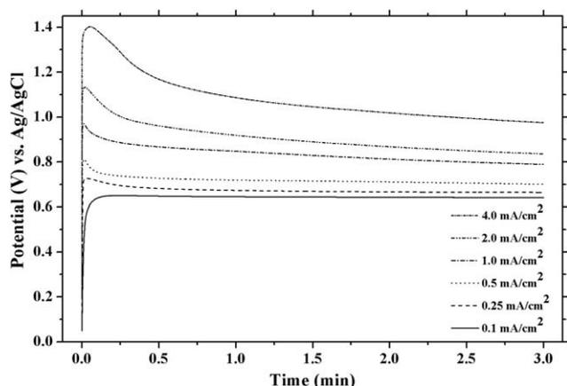
**Fig. 1** Chronopotentiograms over the first 3 min of electropolymerisation of PPy/GG electrode coatings at various current densities.
