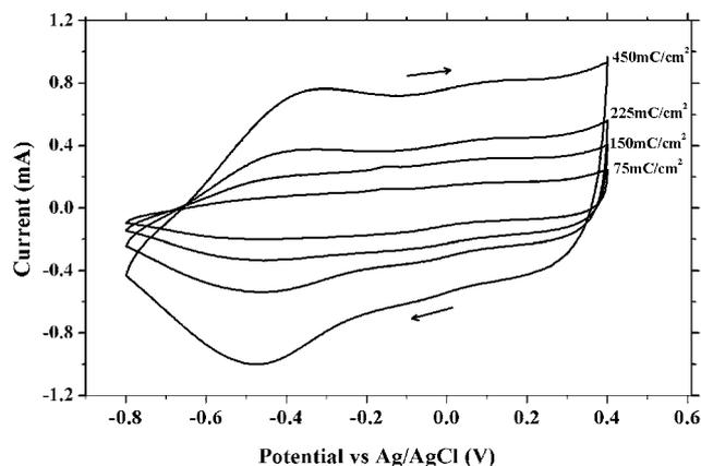
**Fig. 4** Cyclic voltammograms of PPy/GG coated electrodes prepared with polymerisation times of 5, 10, 15 and 30 min at 0.25 mA cm<sup>-2</sup>, equivalent to deposition charges of 75, 150, 225 and 450 mC cm<sup>-2</sup>. The scan rate was 20 mV s<sup>-1</sup>.
