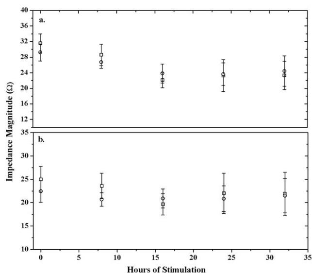
**Fig. 8** Impedance magnitudes of PPy/GG coated electrodes ( $150 \text{ mC cm}^{-2}$ ) at (a) 250 Hz and (b) 1000 Hz, measured at 8 h intervals during biphasic pulsed current stimulation (squares) with comparison to unstimulated controls (circles).
