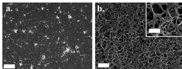
**Fig. 3** SEM images of PPy/GG coatings on Au Mylar substrates polymerised at 0.25 mA cm<sup>-2</sup>. The deposition charges were 37.5 mC cm<sup>-2</sup> (a) and 150 mC cm<sup>-2</sup> (b). Scale bars in (a) and (b) represent 1 μm, and 500 nm for the inset.
