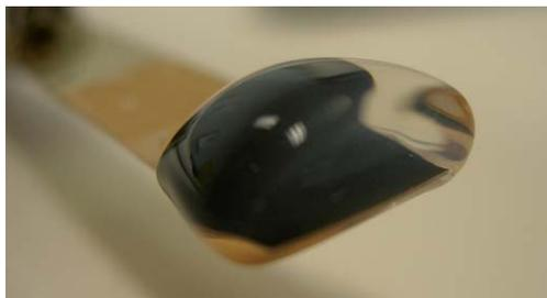
**Fig. 2** Optical image of a PPy/GG coated electrode indicating the secondary GG hydrogel layer on top of the PPy/GG layer when current densities greater than 1 mA cm<sup>-2</sup> were used.
