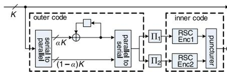
Fig. 1 Encoder of precoded turbo code
