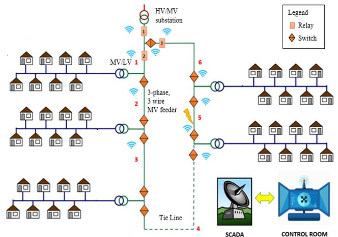
Figure 1. Structure of the automated protection system
