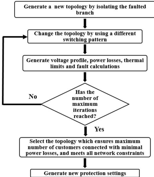
Figure 2. Flow diagram of the proposed algorithm
