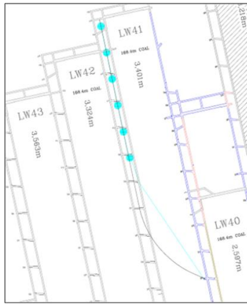
Figure 13 - Plan - proposed borehole MG40-30-1
