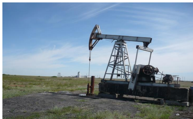
Figure 2 - Nodding donkey pump, with gas flare, with mine Kazakhstanskaya boundary shaft in background
