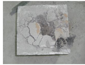
Figure 13 - Fragmentation pattern (25 MPa)
