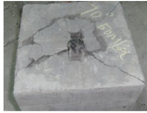
Figure 12 - Fragmentation pattern (50 MPa)
