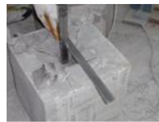
Figure 6 – Measuring the cavity depth
