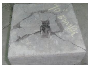
Figure 10 - Fragmentation pattern (50 MPa)
