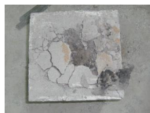
Figure 11 - Fragmentation pattern (25 MPa)
