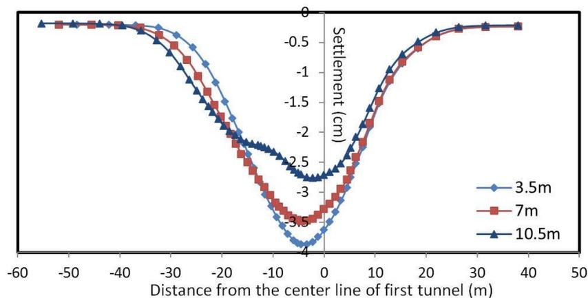
Figure 5 - Surface settlement for different pillar width between tunnels in section 2
