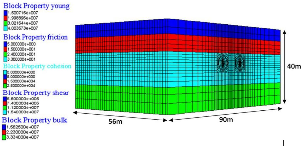
Figure 2 - The mesh used for modelling
