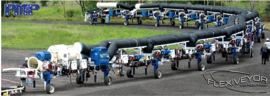
**Figure 1 - Flexiveyor linear mining system (Diversified Mining Services 2010) flexible belt conveyor**
