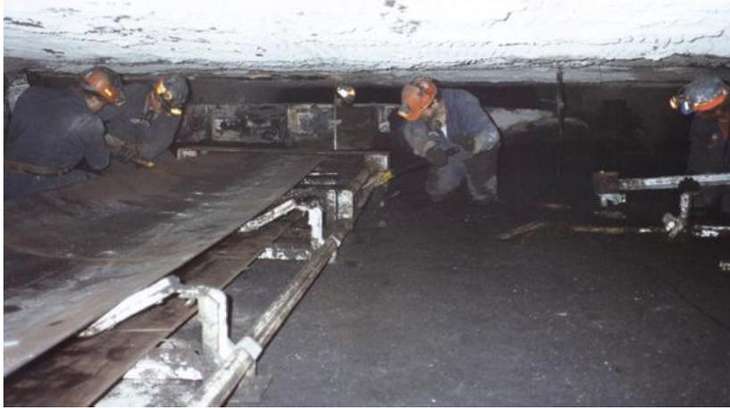
Figure 4 - Temporary belt support (S and S Sliders, 2011)
