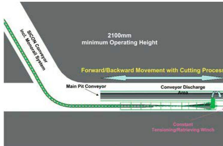
Figure 6 - Vach 500 discharge area (Sandvik, 2010)
