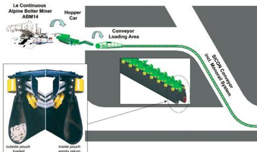
Figure 5 - Vach 500 loading area (Sandvik, 2010)
