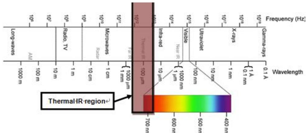
**Figure 4 - The full electromagnetic spectrum, showing the wavelengths associated with thermal infrared energy. For comparison, the familiar visible light spectrum is also shown. (Courtesy L. Keiner, Coastal Carolina University, adapted).**
