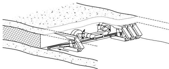
**Figure 1 - Representation of a small portion of a longwall operation. The coal seam is indicated by the hatched layer between the underlying and overlying strata. For clarity, the central section of the roof support system is not shown.**
