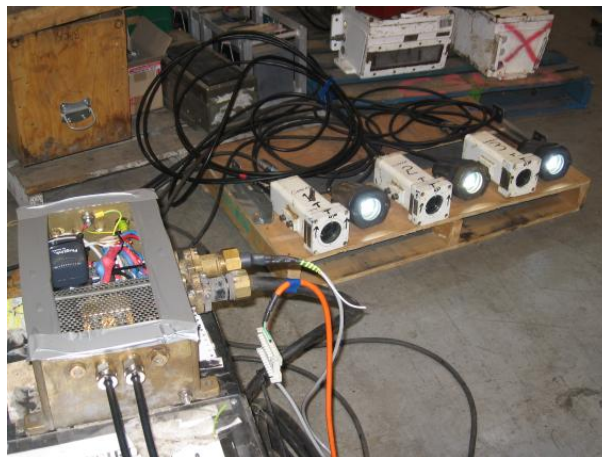
Figure 3 - In-house validation of a three-camera visible light camera system. To the left of the image is the junction box which houses the communications components, and to the right are the cameras and lighting flameproof enclosures.
