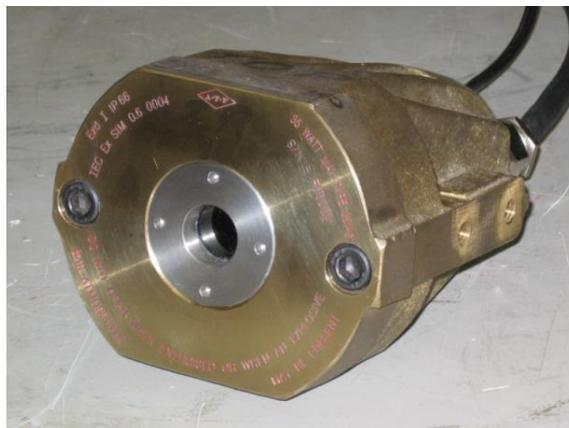
**Figure 6 - An approved TIR thermal infrared flameproof enclosure and camera conforming to IEC Ex d standards**
