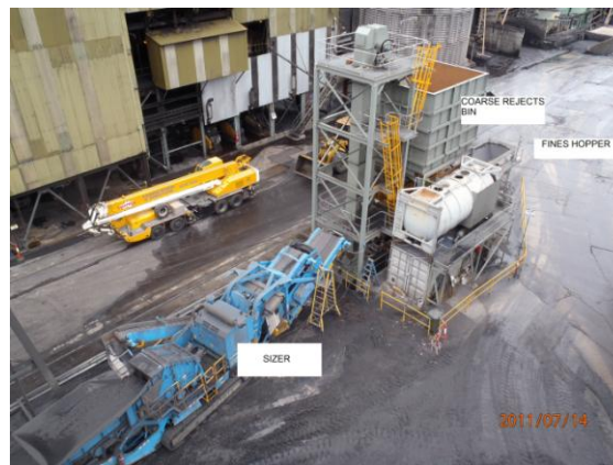
Figure 8 - Pilot plant layout
