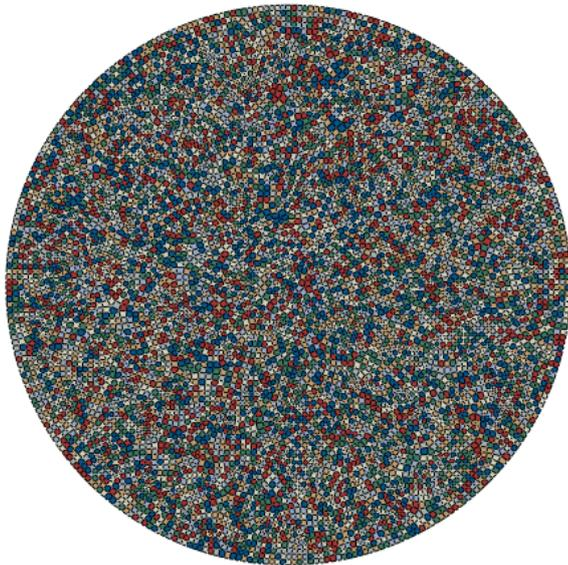
**Figure 1.** Voronoi diagram of blank with 49555 grains
