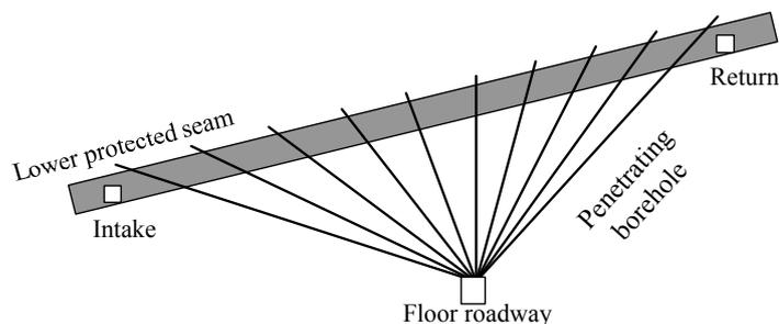
**Figure 4 - Layout inclination diagram of the grid-type penetrating borehole in floor roadway**
