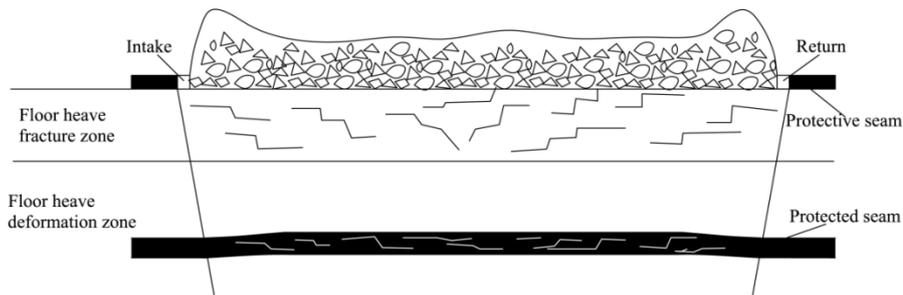
Figure 2 - Fracture zones of floor stratum
