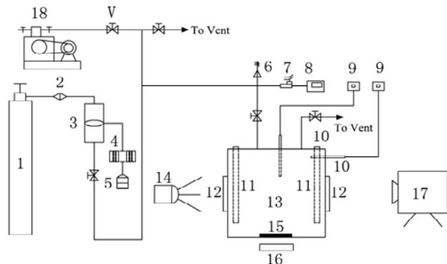
1 - gas cylinder; 2 - filter; 3 - booster pump; 4 - frozen compressed air dryer; 5 - air compressor; 6 - safety valve; 7 - pressure sensor; 8 - pressure digital display instruments; 9 - temperature display instruments; 10 - thermocouple; 11 - electric heat bar; 12 - visual transparent window; 13 - visual cell; 14 - light; 15 - magneton; 16 - electromagnetic stirrer; 17 - rapid imaging system; 18 - vacuum pump; V - cut-off valve
