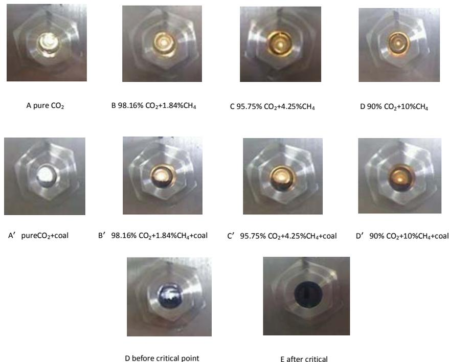
Figure 6 - Pictures of critical points of different components of the CO<sub>2</sub>-CH<sub>4</sub> binary system and CO<sub>2</sub>-CH<sub>4</sub>+coal system
