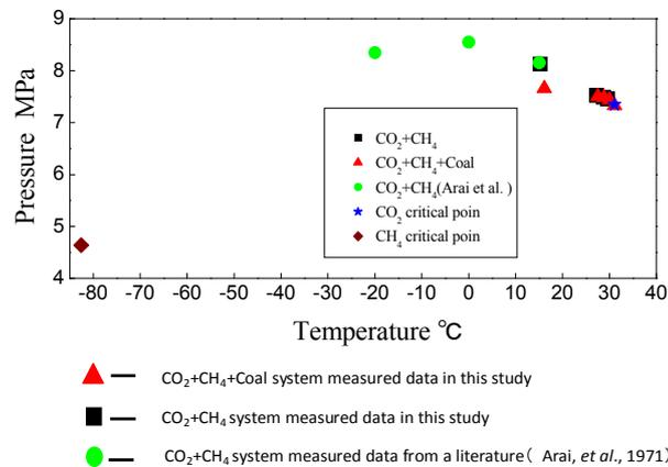
Figure 5 - The supercritical parameters of the CO<sub>2</sub>-CH<sub>4</sub> system
