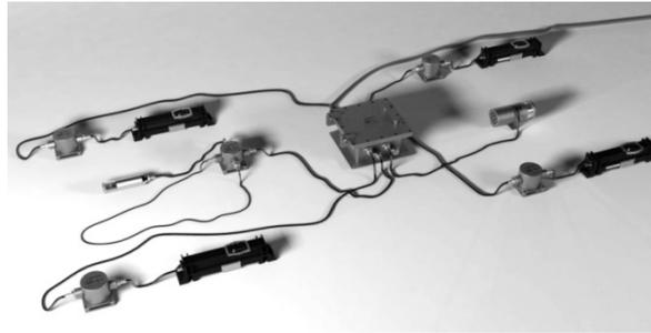
**Figure 3 - HazardAvert on-machine components**
