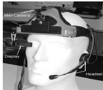
**Figure 2 - BMW AR system (after Platonov *et al.*, 2006)**
