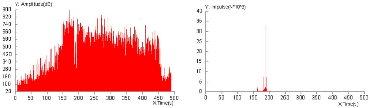
Figure 6 - Changes in AE amplitude and impulse with time (Channel 7-150 kHz)
