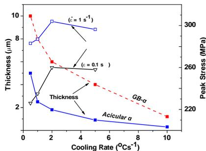
**Figure 2.** The thickness of  $\alpha$ -phases and peak stress as functions of cooling rate
