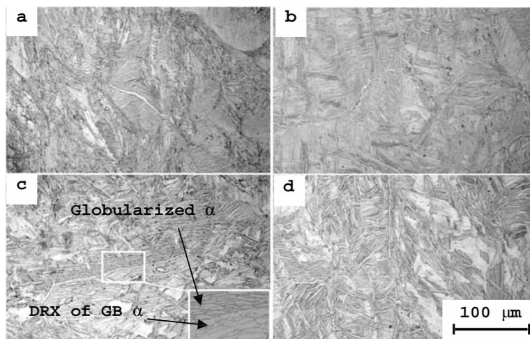
**Figure 4:** The microstructure of Ti64 alloy deformed at 1073 K after cooling at different rates of **a)**  $5 \text{ ks}^{-1}$ , **b)**  $2 \text{ ks}^{-1}$ , **c)**  $1 \text{ ks}^{-1}$  and **d)**  $0.5 \text{ ks}^{-1}$  ( $\dot{\epsilon} = 1 \text{ s}^{-1}$ )
