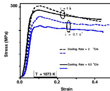
**Figure 3.** The flow curves of samples deformed at 1073 K at different strain rates
