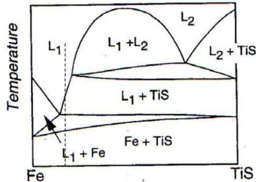
Figure 8: Schematic phase diagram of TiS pseudo-binary system<sup>20</sup>
