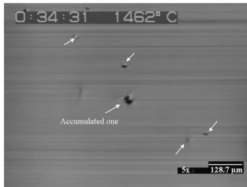
Figure 3: Floating particles on the surface of liquid steel during heating
