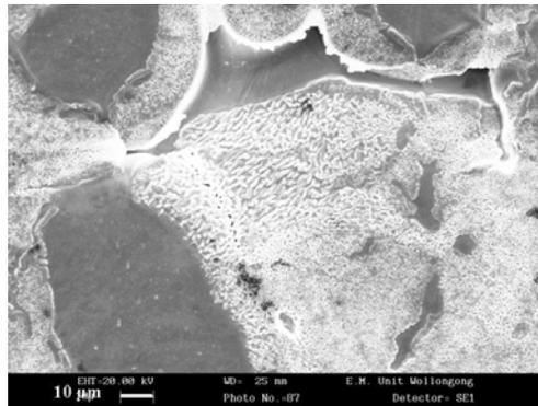
Figure 6: SEM photograph of a colony of precipitates
