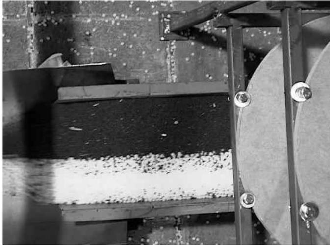
**Figure 5** Top View of Segregated Materials (Plastic Pellets and Canola Seed) Being Discharged from Twisted Standpipe
