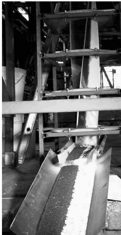
**Figure 6** End View of Segregated Materials (Alumina Hydrate [White Material] and Canola Seed) Being Discharged from Twisted Standpipe
