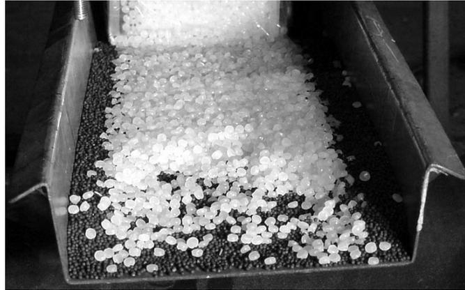
**Figure 3** Vibrating feeder
