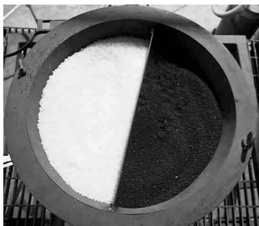
**Figure 2** Top View of Feeding Hopper Showing the Partition Separating the Feed Materials
