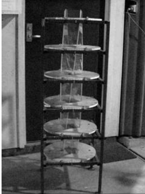
**Figure 1** Test Rig with Approximately 90° Twist Imposed on the Perspex Tube
