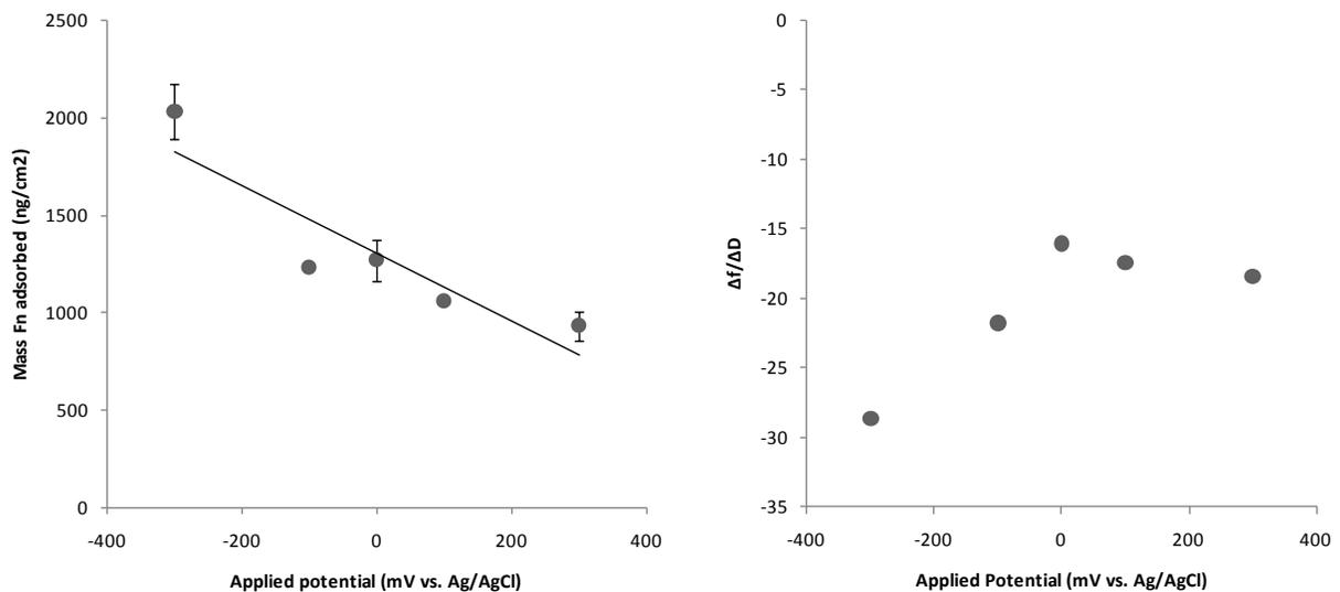
**Figure 5.** Properties of the fibronectin protein layer adsorbed to the 48 wt.-% PEDOT surface a) Representation of the trending change in adsorbed mass as a function of charge applied. Means represent the average of two samples and error bars represent the range. b) Changes in mechanical properties as a function of charge applied represented by the  $\Delta f/\Delta D$  ratio.
