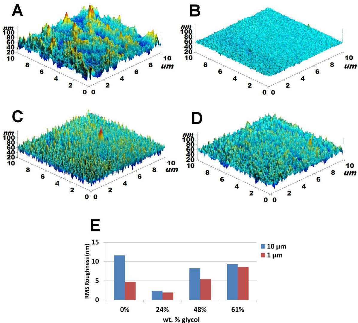
**Figure 3.** AFM topography images for samples made with: A) 0%; B) 24%; C) 48% and; D) 61% glycol in oxidant layer. E) The RMS roughness measured at length scales of 1 and 10  $\mu\text{m}$  (Note:  $\text{RMS}_{\text{std dev.}} < 10\%$  relative for all samples and measured scan areas)
