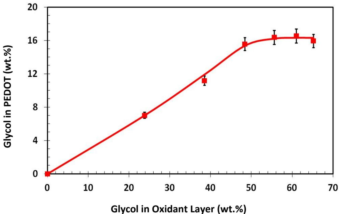
**Figure 2.** Weight percentage of glycol surfactant within the PEDOT polymer as a function of the glycol content in the oxidant layer.
