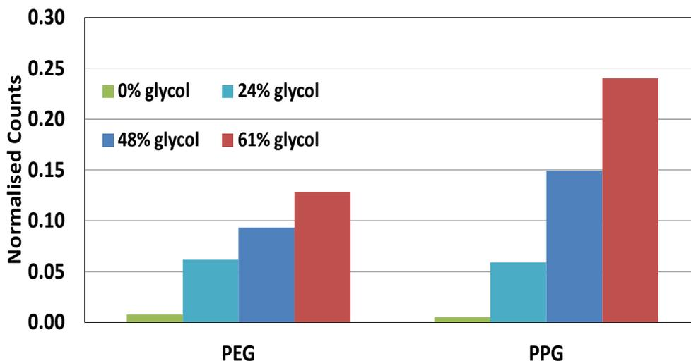
**Figure 4.** ToF-SIMS relative measurements of the PEG and PPG moieties in the glycol surfactant, which now resides within the PEDOT polymer surface (*i.e.* top 1-2 nm) for the different glycol weight percents originally in the oxidant layer. (95% confidence level with N = 10 samples)
