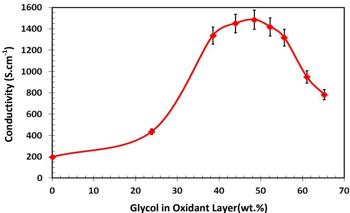
**Figure 1.** VPP PEDOT conductivity as a function of weight percentage of the glycol surfactant within the oxidant layer. (Glycol content within PEDOT capped at 16 wt.%, See Fig. 2)
