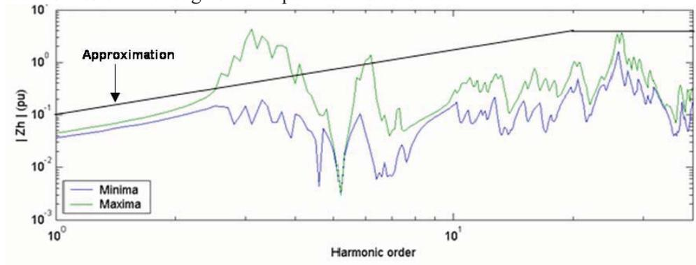
**Figure 4: Harmonic impedance variation and approximation of (9)**
