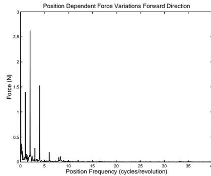
Figure 9: Linear Motor Frequency Spectrum
