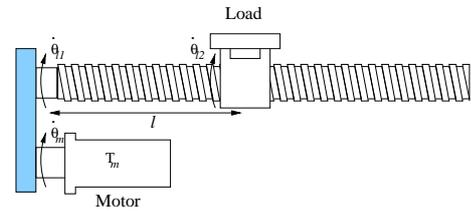
Figure 3: Diagram of a Belt Driven Ball Screw
