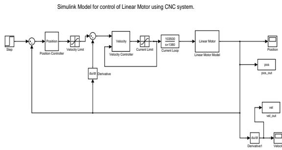
Figure 4: Simulink Model for Linear Motor System
