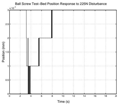
Figure 8: Ball Screw Axis Position (225N Disturbance)
