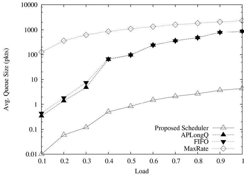
Figure 5: Queue size versus load. In this experiment, there are 10 APs and 20 stations. Each arrival contains a burst size of five packets.
