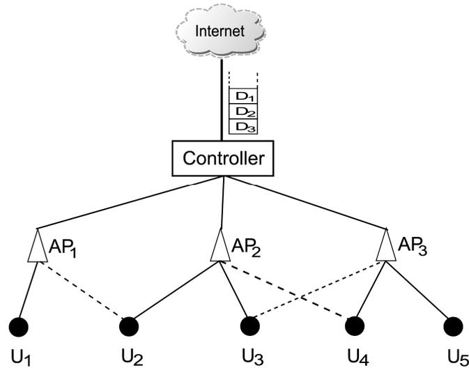
Fig. 1: An example enterprise WLAN with three APs.  $u_x$  denotes station  $x$ . Solid line indicates the associated AP of a given station. Dotted lines indicate alternate APs that can be used to deliver packets to stations.  $D_x$  corresponds to a data packet for station  $x$ .
