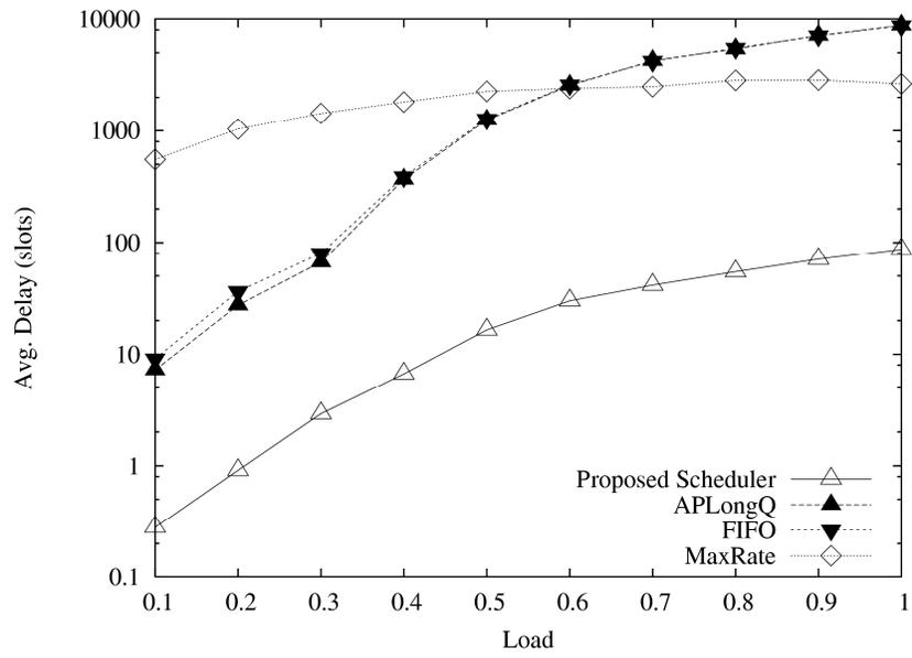
Figure 4: Load versus delay. 10 APs and 20 stations. Burst size fixed at five packets.
