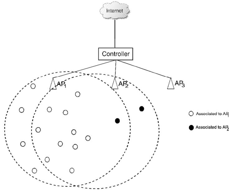
Figure 2: An example where most stations are associated to AP<sub>1</sub>. This means AP<sub>1</sub> will have the highest load. A better option is to have AP<sub>2</sub> help forward packets to stations associated to AP<sub>1</sub>.
