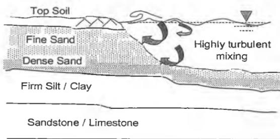
Fig. 2 Typical Layers of Coastal Soils due to Million Years of Geological Deposition
