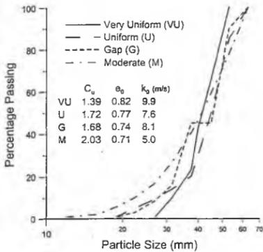
Fig. 22 Particle Size Distributions Used in Triaxial Tests, along with their Uniformity Coefficients,  $C_u$ , Initial Void Ratios,  $e_0$  and Permeability Coefficients,  $k_0$  (Indraratna et al., 2004)
