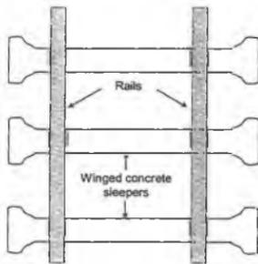
Fig. 29 Sleepers with Enlarged Ends to Increase the Confining Pressures
