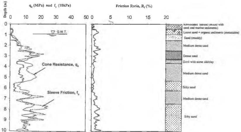
Fig. 7 Cone Penetration Test Results of Soil Layers (CPT) after Tsunami Occurrence (Site 1)
