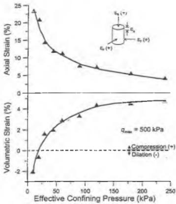
Fig. 26 Variation of Axial and Volumetric Strains with Confining Pressure (Indraratna et al., 2005)
