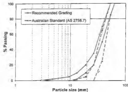
Fig. 25 Recommended Railway Ballast Grading in Comparison with the Current Australian Standard Grading Requirements (Indraratna et al., 2004)
