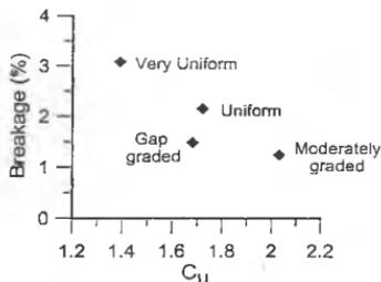
Fig. 24 Effect of Grading on Particle Breakage (Indraratna et al., 2004)
