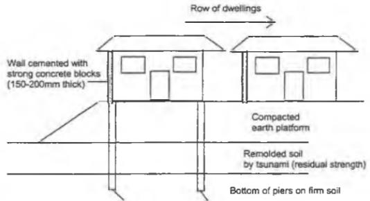
Fig. 11 Housing Construction on Raised Earth Platform
