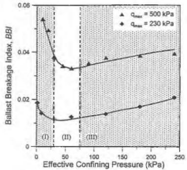
Fig. 27 Effect of Confining Pressure on Particle Degradation (Indraratna et al., 2005)
