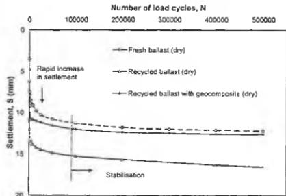
Fig. 19 Settlement of Fresh Ballast and Recycled Ballast with and without Geosynthetics (dry samples)
