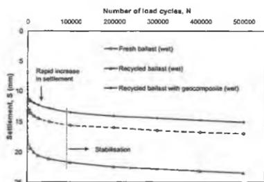
Fig. 20 Settlement of Fresh Ballast and Recycled Ballast with and without Geosynthetics (Wet Samples)
