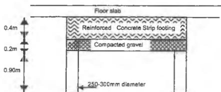
Fig. 13 Foundation for Soils Affected by Tsunami (Section A-A)
