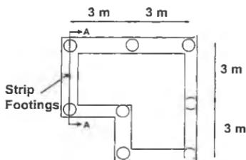
Fig.14 Typical Plan View of Foundation Construction
