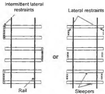
Fig. 30 Increasing Confining Pressure Using Intermittent Lateral Restraints
