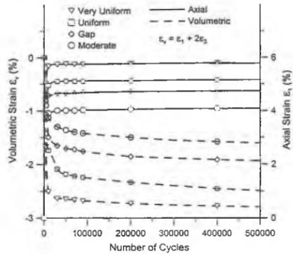
Fig. 23 Axial and Volumetric Strain Response of Different Distributions under Cyclic Loading (Indraratna et al., 2004)
