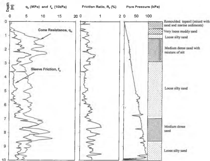
Fig. 8 Cone Penetration Test with Pore Pressure Measurement Results (CPTU) of Soil Layers after Tsunami Occurrence (site 2)
