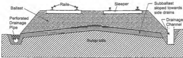
Fig. 17 Schematic Illustration of Track Drainage System (after Selig and Waters, 1994)
