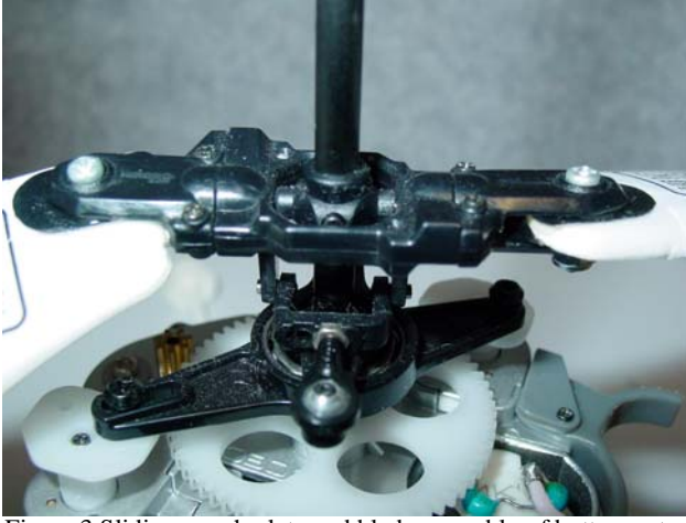
Figure 3 Sliding swash plate and blade assembly of bottom rotor
