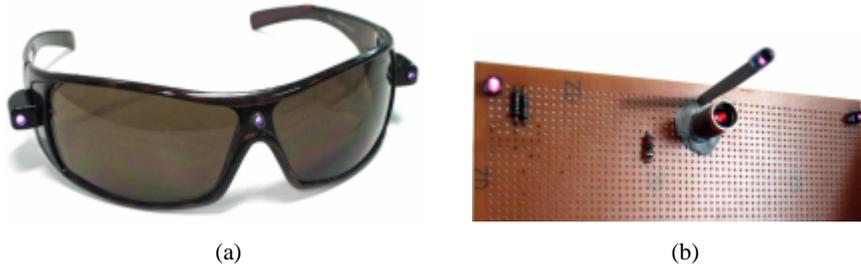
**Figure 1.** (a) Prototype LED Spectacles (b) LED testing hardware
