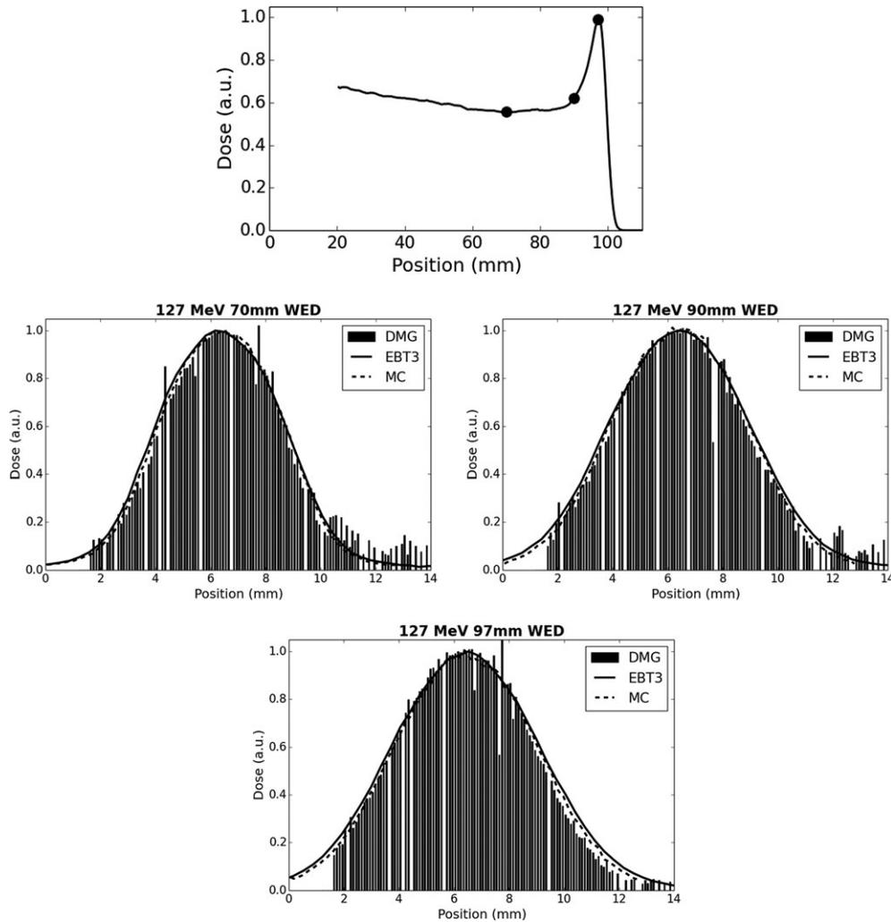
**Fig. 8.** Measured beam profiles at varying depths in water for a 127 MeV proton beam. Geant4 simulation data are also provided for comparison. A simulated central beam axis depth dose profile utilizing  $0.25 \times 0.25 \times 0.25 \text{ mm}^3$  voxels with DMG measurement locations marked is provided for reference (top).
