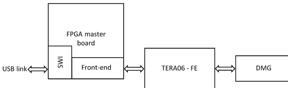
Fig. 3. DMG data acquisition architecture.
