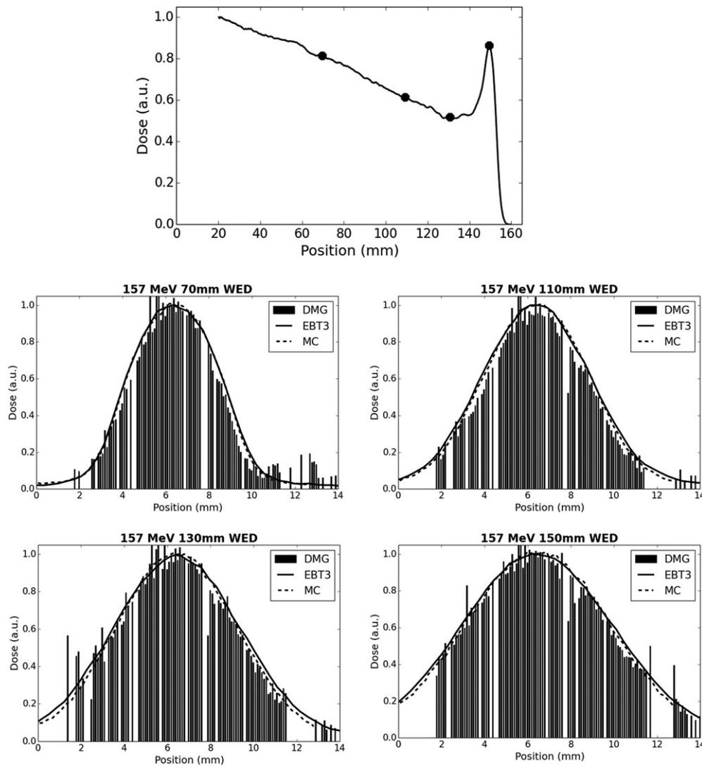
**FIG. 9.** Measured and simulated beam profiles at varying depths in water for a 157 MeV proton beam. Geant4 simulation data are also provided for comparison. A simulated central beam axis depth dose profile utilizing  $0.25 \times 0.25 \times 0.25 \text{ mm}^3$  voxels with DMG measurement locations marked is provided for reference (top).
