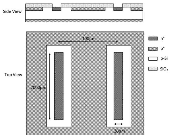
**Fig. 1.** Schematic of two n<sup>+</sup> SV elements in the DMG detector. Note the entire DMG is comprised of 128 SV elements.
