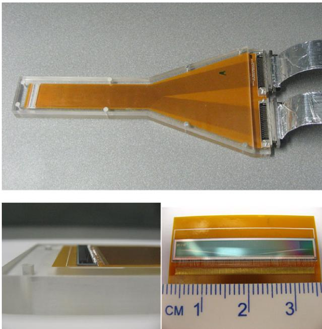
**FIG. 2.** Images of the DMG probe used in this work. The minimal thickness (lower left) allows for a wide range of mounting options and minimal perturbation of the proton beam while the linear array (lower right) allows for concurrent point dose and beam profile measurements.
