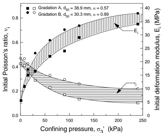
**Figure 5 Influence of cell pressure on initial deformation modulus and Poisson's ratio in initial loading stage (Indraratna et al, 1998)**
