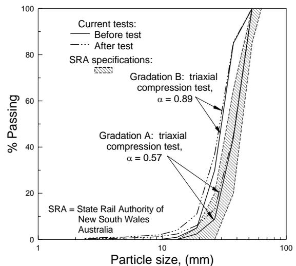
**Figure 1 Particle size distribution of Latite Basalt (SRA, 1983; Indraratna et al, 1998)**
