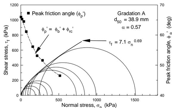
Figure 7 Mohr-Coulomb failure envelopes for Latite Basalt (Indraratna et al, 1998)
