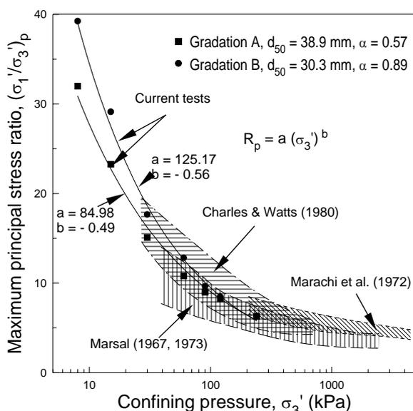
**Figure 6 Influence of confining pressure on principal stress ratio at peak for Basalt in comparison with various granular media (Indraratna et al, 1998)**
