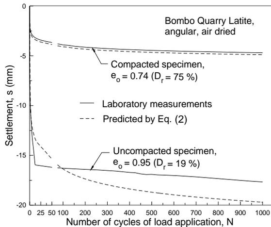
**Figure 14 Effect of load cycles on settlement upon repeated loading**
