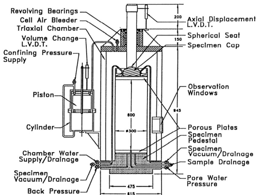
**Figure 2 Large scale triaxial equipment**
