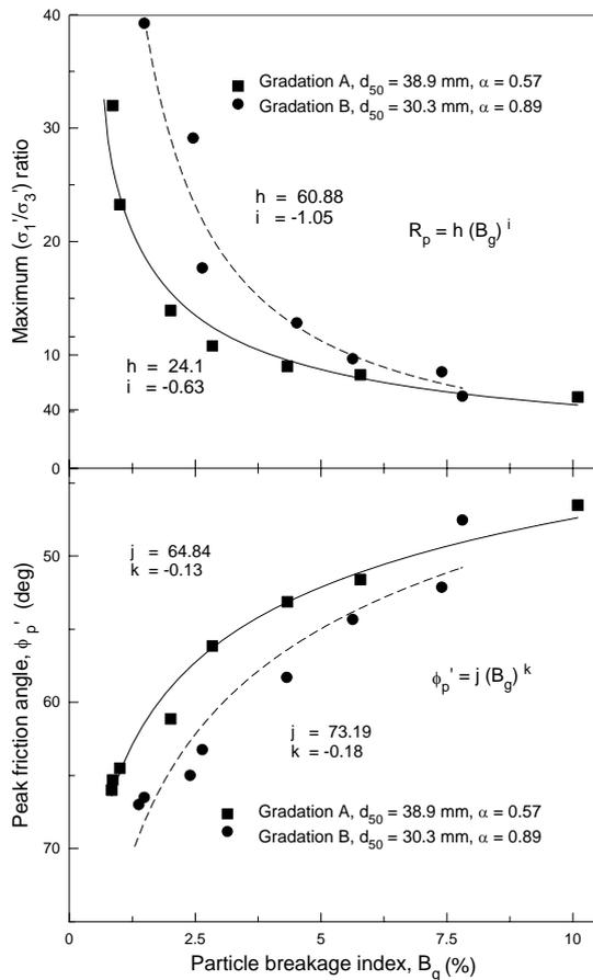
**Figure 10 Effect of stress variation on particle breakage for Bombo Basalt (Indraratna et al, 1998)**
