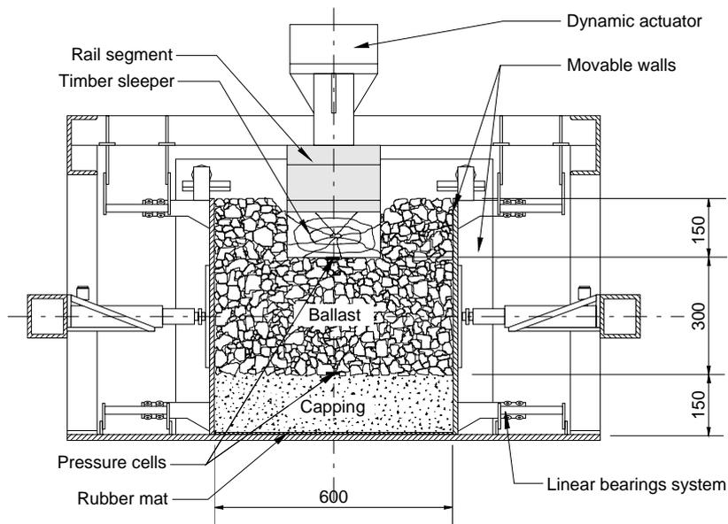
Figure 15 Cubicle triaxial testing rig with dynamic loading
