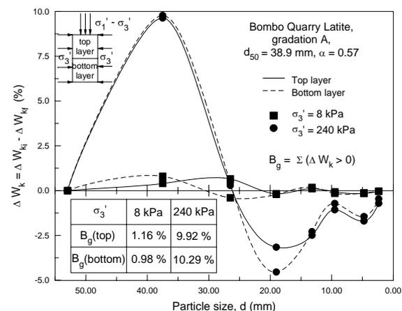
Figure 9 Variation of particle distribution with grain size for Bombo Basalt sheared at different confining pressures (Indraratna et al, 1998)
