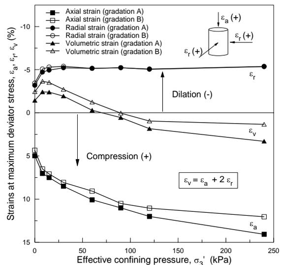
**Figure 4 Variation of sample strains at peak deviator stress with confining pressure and grain size (Indraratna et al, 1998)**
