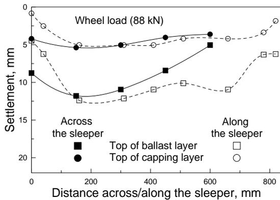
Figure 17 Settlement of ballast and capping layers in the cubicle rig
