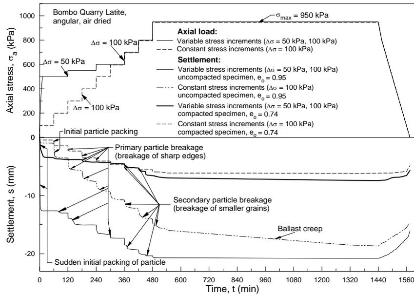
Figure 12 Settlement-time response for ballast, indicating particle breakage (Indraratna et al, 1997)
