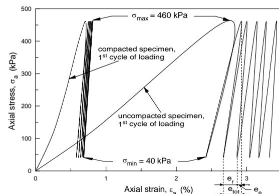
Figure 13 Stress-strain behaviour of loose and dense ballast under repeated loading unloading
