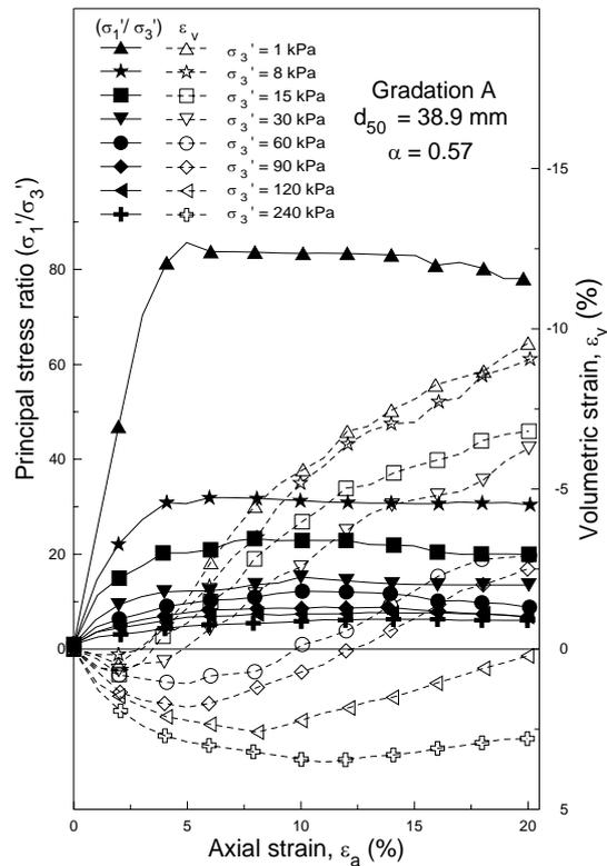
**Figure 3 Drained compression tests at different confining pressure values on Latite Basalt (Indraratna et al, 1998)**
