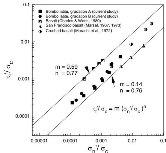
Figure 8 Normalized shear strength-normal stress relationship for various aggregates (Indraratna et al, 1998)
