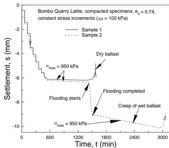
Figure 19 Effect of wetting on ballast settlement
