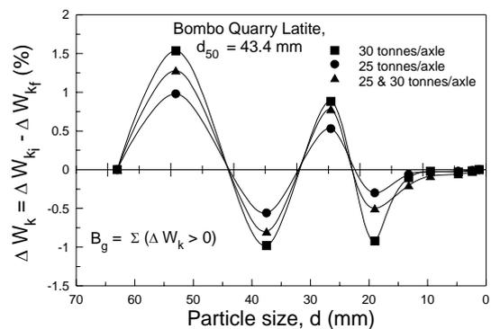
Figure 18 Grain breakage in dynamic triaxial testing
