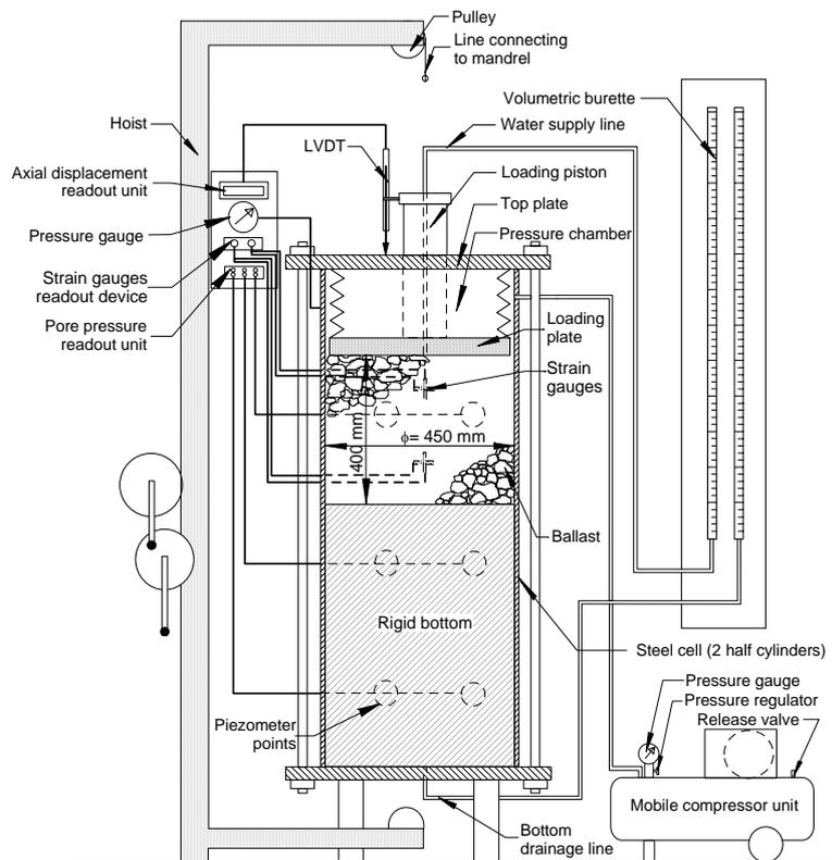
**Figure 11 Large scale consolidometer for testing ballast**
