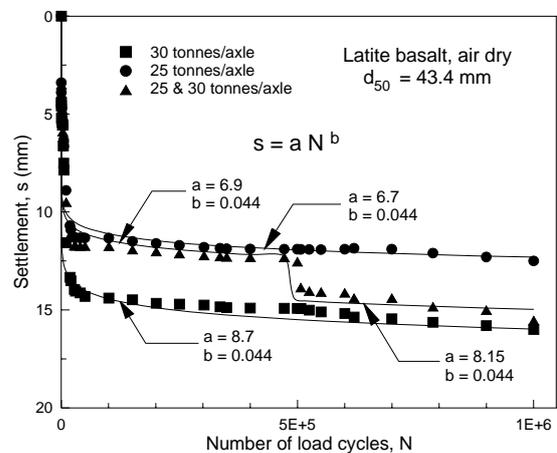
Figure 16 Effect of load cycles and axle loads on settlement
