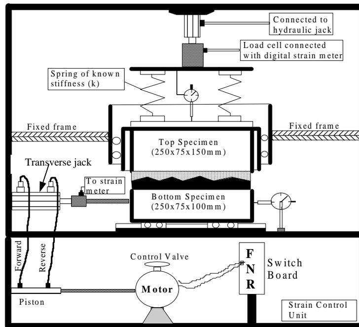
Figure 1. Schematic diagram of the CNS shear apparatus (Indraratna et al. 1998).
