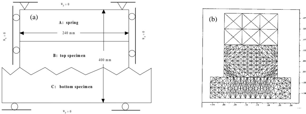
Figure 2. (a) Conceptual model for laboratory CNS shear behaviour and (b) discretisation of blocks
