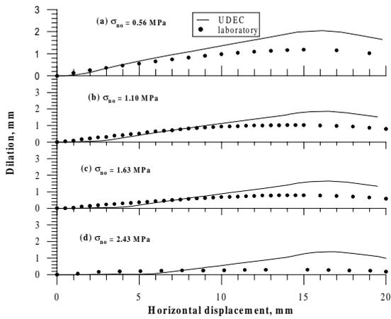
Figure 4. UDEC prediction and observed dilation behaviour of Type I joint under CNS.
