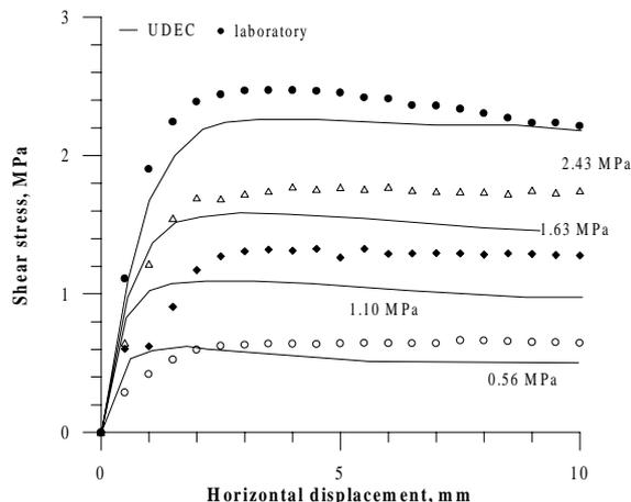
Figure 6. UDEC prediction and laboratory shear behaviour of Type I joint under CNL.
