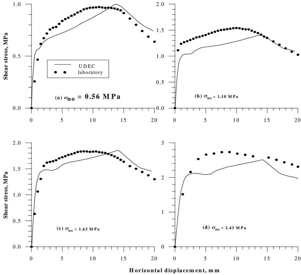
Figure 3. UDEC prediction and observed shear stress responses for Type I joints under CNS.
