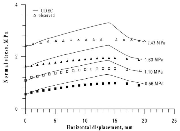
Figure 5. UDEC prediction and observed normal stress responses for Type I joint under CNS.
