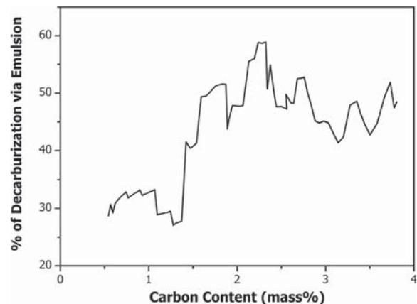
Fig. 5. Carbon removal via emulsion calculated by the model and based on the operating conditions described by Cicutti *et al.*<sup>22)</sup>
