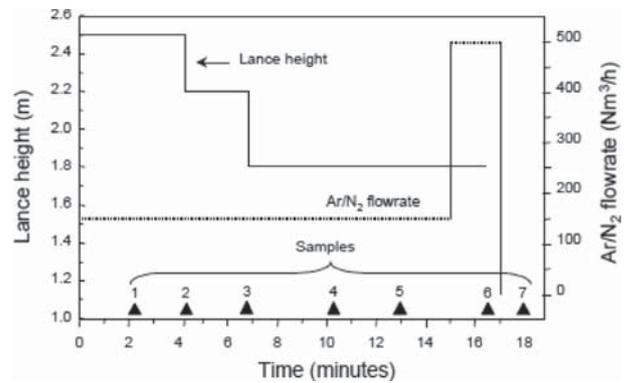
**Fig. 2.** The variation in lance height, inert gas flow rate and sampling point during the blowing process.
