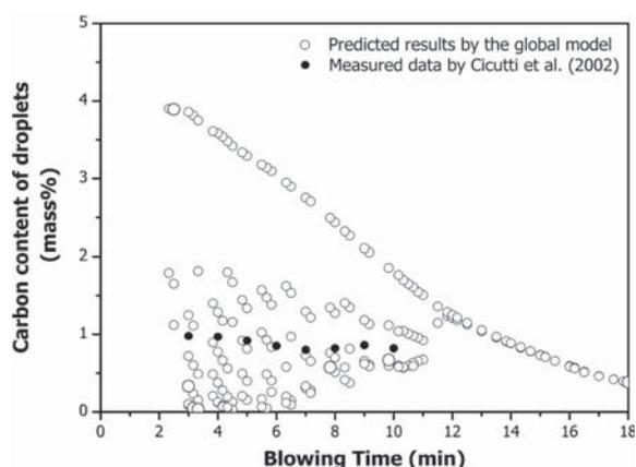
Fig. 10. Comparison of carbon content in metal droplets predicted by the proposed model with the measured carbon content of metal droplets reported by Cicutti *et al.*<sup>22)</sup>
