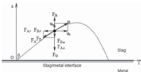
**Fig. 1.** The schematic illustration of ballistic motion of a metal droplet in slag.<sup>20)</sup>
