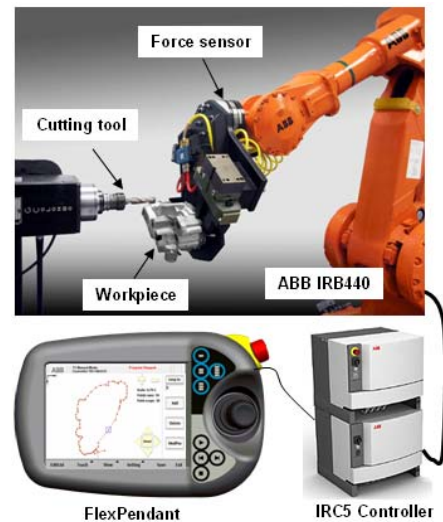
Figure 1. System Setup for Robotic Machining with Force Control
