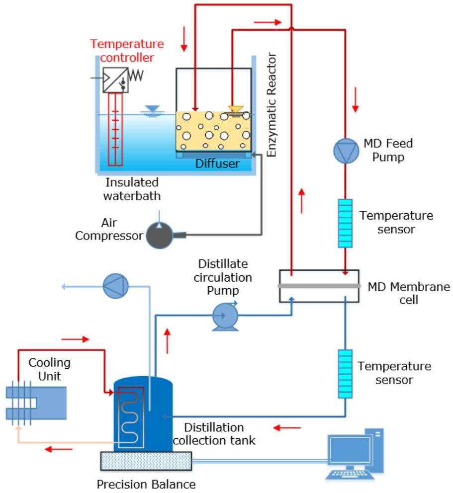
**Figure S1.** Schematics of membrane distillation-enzymatic membrane bioreactor (MD-EMBR)
