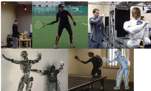
Fig. 1. Vicon motion capture system. Cameras in corner of room (red lights), markers on the actors body [35]. Xsens Moven [13]. On the right is robot imitation with inertial sensors [23]. Below right is the SARCOS robot imitate person in mechanical motion suit and below left is a hybrid inertial and acoustic motion suit [37].
